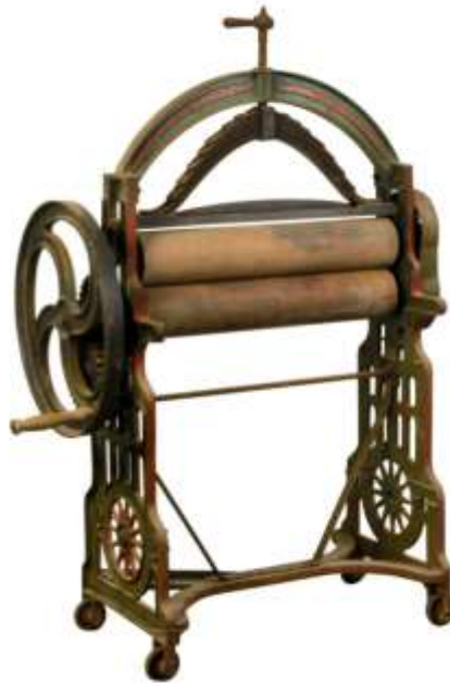
Large wringer on casters, entirely in metal. The pressure level varied with the tightening of the knob at the top of the frame.
