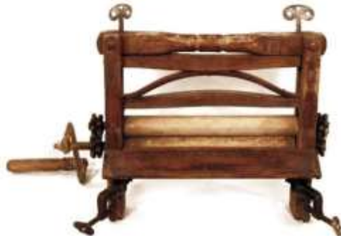
Manual wringer fitted to a receptacle or a washing machine using a system of clamps. The pressure exerted on the laundry was regulated using two wing nuts on either side of the wooden frame above a metallic hanger.
